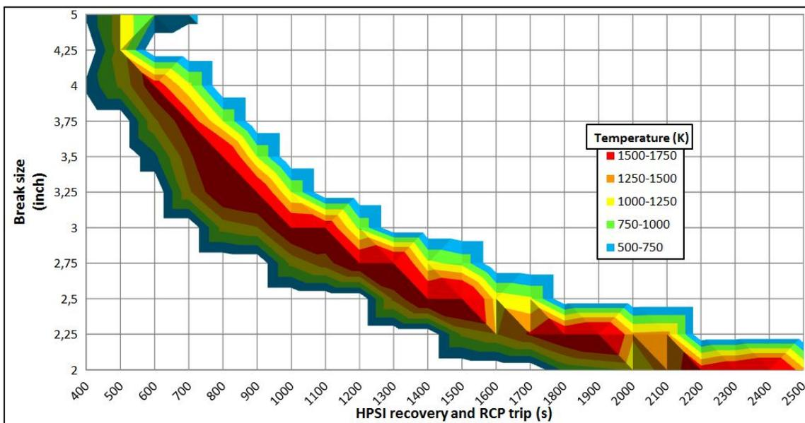
Figure 29: PCT for different break sizes and HPSI recovery and 3/3 RCP trip times.
