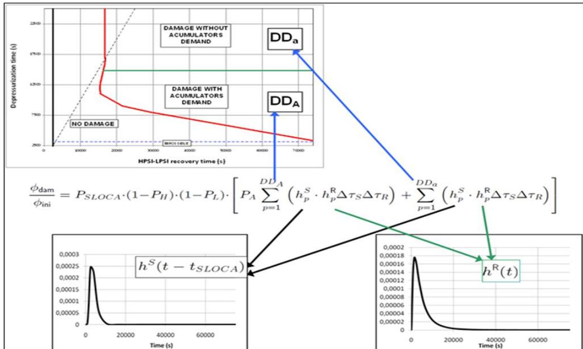
Figure 17. TSD procedure of calculating the PCT exceedance frequency.
