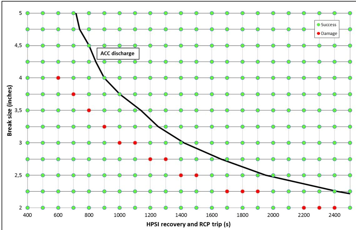
Figure 28: Damage Domain obtained for different break sizes and HPSI system recovery/RCP trip times.
