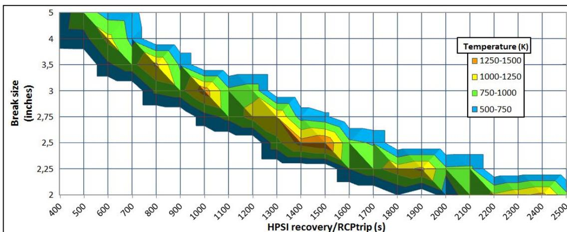
Figure 31: PCT for different break sizes and HPSI recovery and 2/3 RCP trip times (RCP broken loop is kept off).
