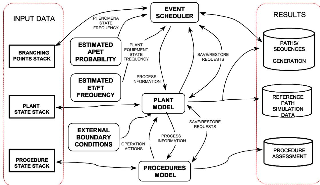
Figure 5. ISA/SCAIS elements for Automatic Generation of Paths and Sequences.
