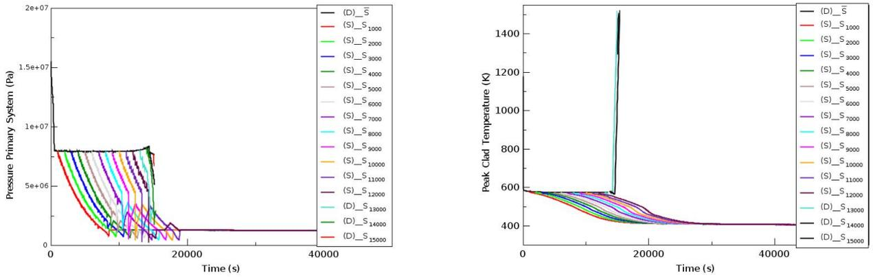
Figure 23. RCS Pressure and PCT in Path Analysis LOCA 1". (Sequence h - S(t) - (0/3A) - L)
