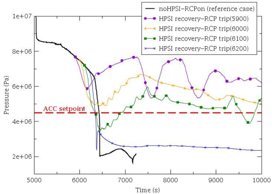
Figure 26: RCS pressure for 3 inch SBLOCA. HPSI recovery and simultaneous 3/3 RCP trip at different times.
