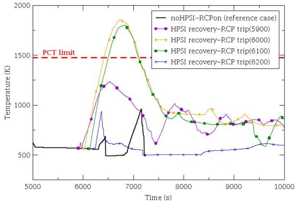
Figure 27: Peak Cladding Temperature for 3 inch SBLOCA. HPSI system recovery and simultaneous 3/3 RCP trip at different times.
