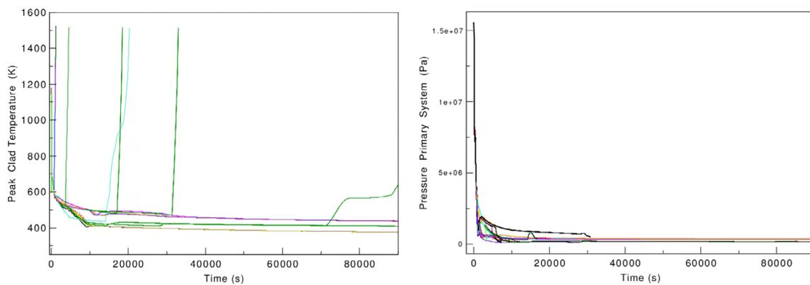
Figure 19. Pressure in RCS and PCT for every sequence of the DET (5 inches) (only 3-ACCUM results are shown in order to simplify the Figures)
