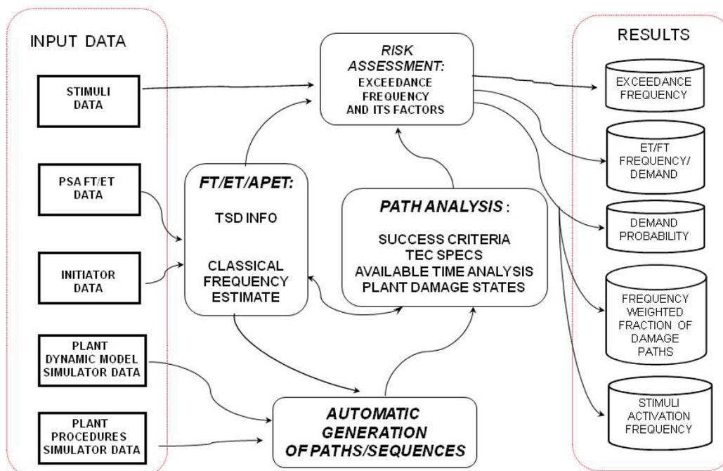
Figure 4. Simplified scheme of the ISA methodology and SCAIS conceptual blocks.
