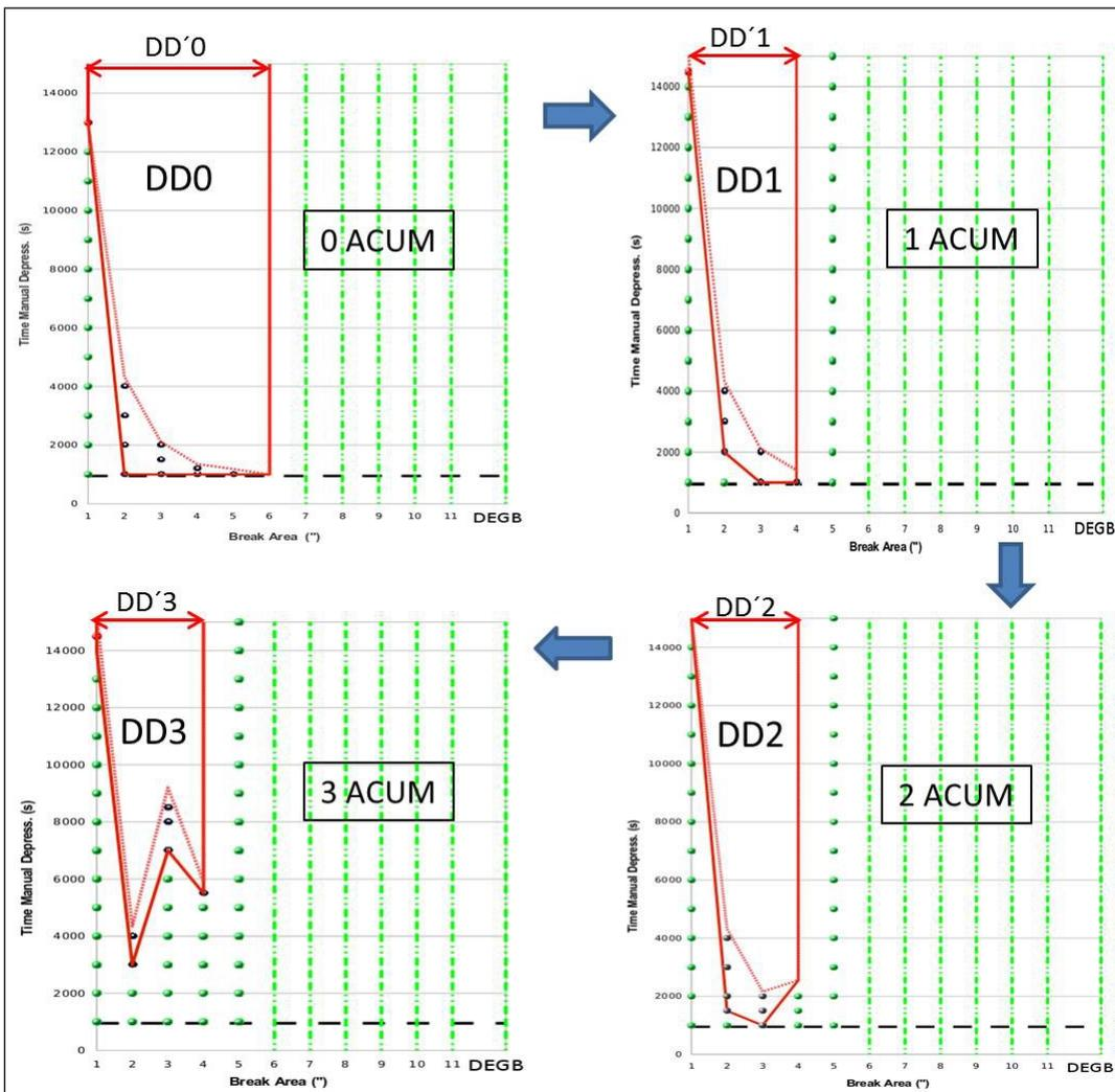
Figure 24. Damage Domains, 0/1/2/3 ACCs available. h-S(t)-(n/3)A-L sequences.
