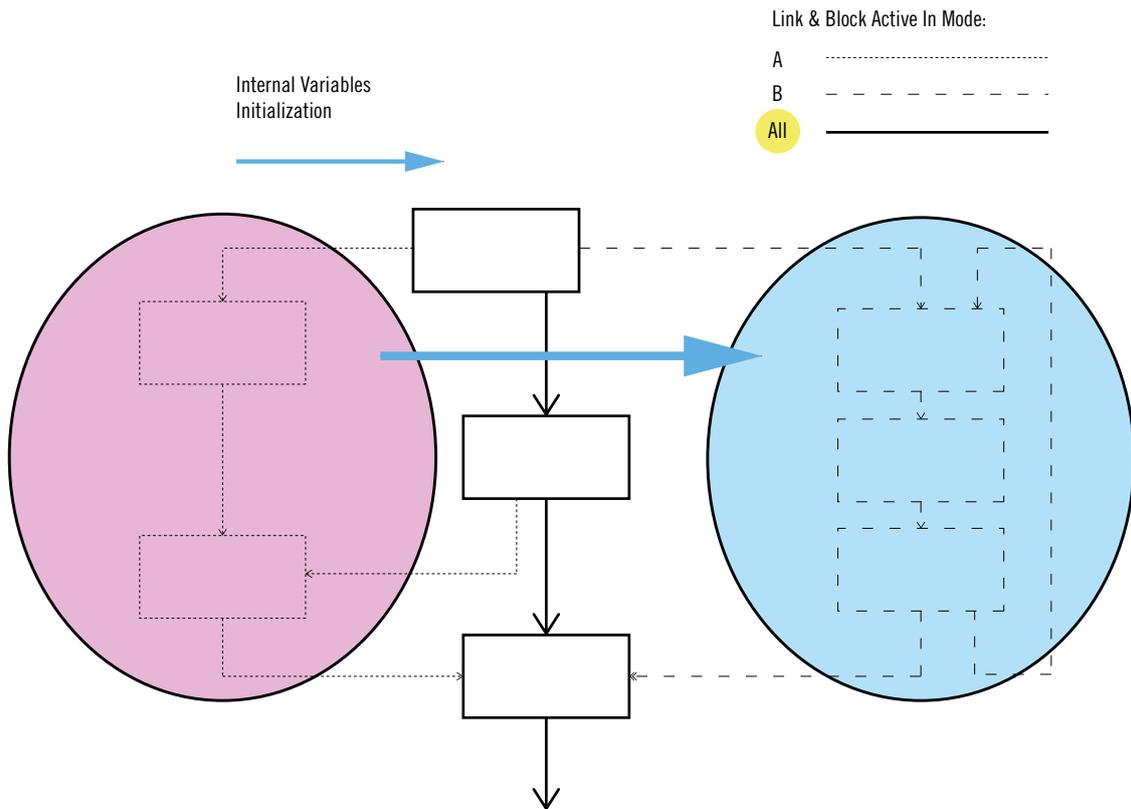
Figure 9: Use of the initial conditions scheme to replace a section of the simulation model.
