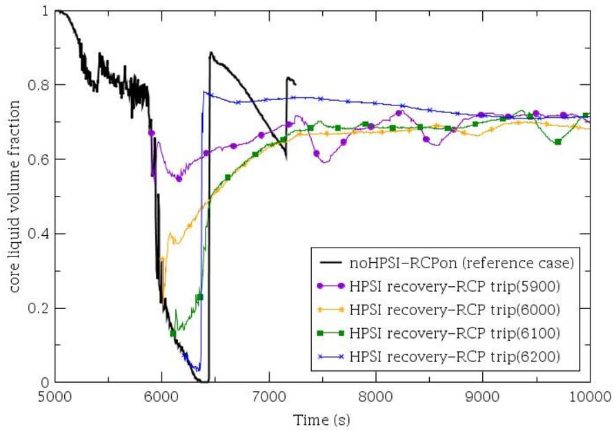
Figure 25: Core level for 3 inch SBLOCA. HPSI recovery and simultaneous 3/3 RCP trip at different times.
