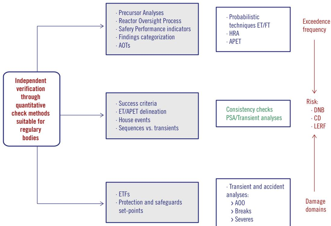
Figure 10. PSA and DSA methods and typical licensing applications.
