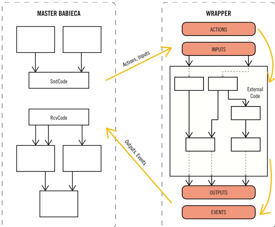
Figure 8: Use of the boundary conditions scheme to connect an external code to BABIECA.
