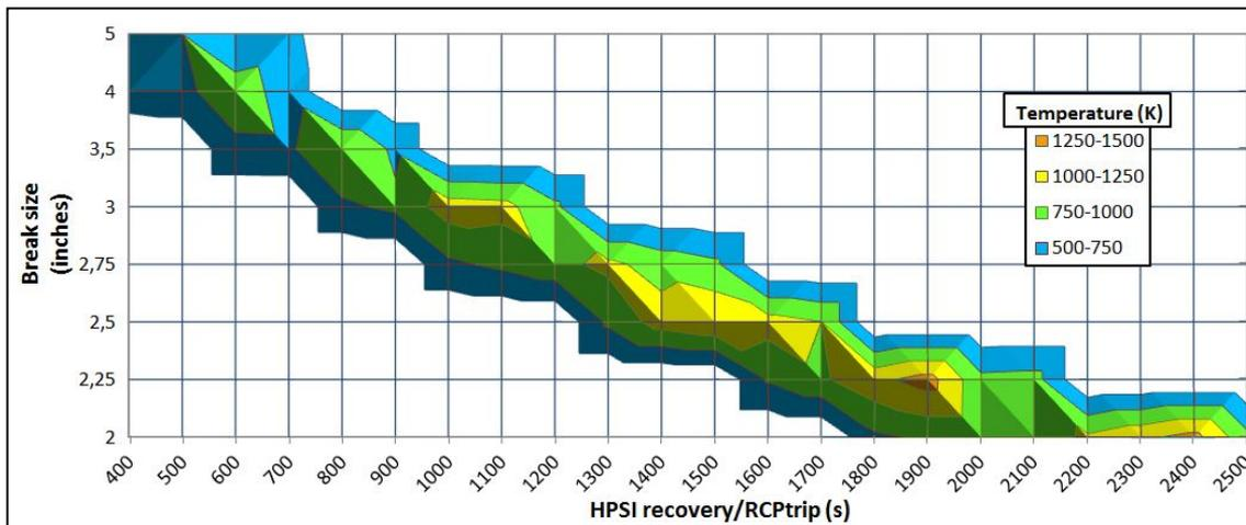
Figure 30: PCT for different break sizes and HPSI recovery and 2/3 RCP trip times (RCP broken loop is kept on).
