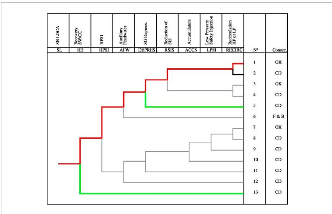
For each seal leakage scenario, the most sensitive sequences to the power uprate were identified. It was found that the sequences with highest impact in PCT always involved failure of HPSI (probability  $2.2E-05$ ). A rough estimation of frequencies based on the Zion PSA data was performed. It was found that the collective frequency of these sequences (sequences 7 to 12 in Figure 8) was about  $8.69E-09$  which clearly falls below the cut-off frequency of  $1E-07$ .
