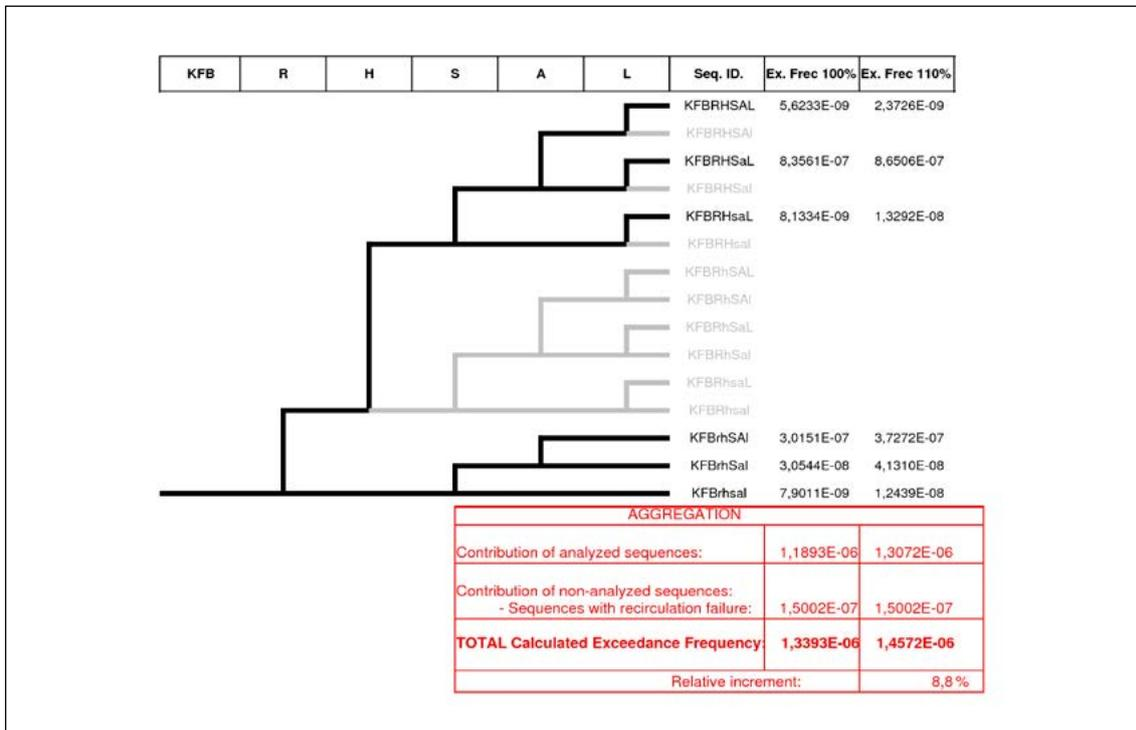
Bold lines in this event tree correspond to the sequences that resulted from the discussion in Section 5.8 above, i.e., the sequences that have been actually quantified. Shadow sequences have not been quantified but are expected to result in negligible contributions.
