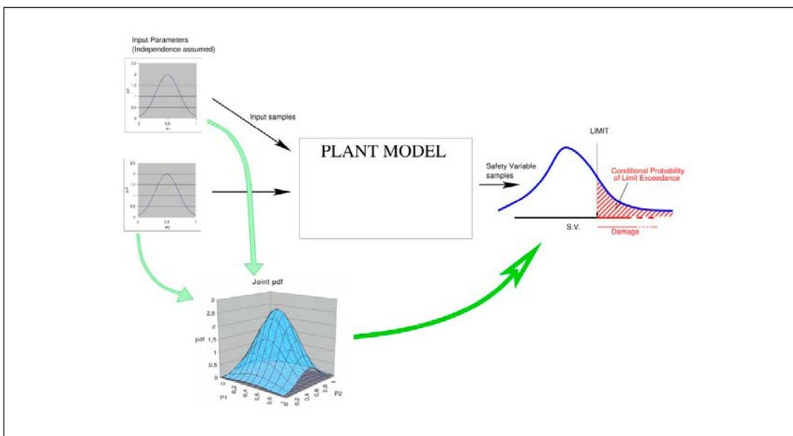
The uncertainty propagation approach is schematically described in Figure 15 for uncertain input parameters only. By sampling input parameters using their probability distributions and using adequate statistical methods, the joint input probability distribution (blue surface in figure 15) is propagated through the simulation model and a distribution of the safety variable can be estimated. The red area under the output distribution represents the conditional probability of limit exceedance.
