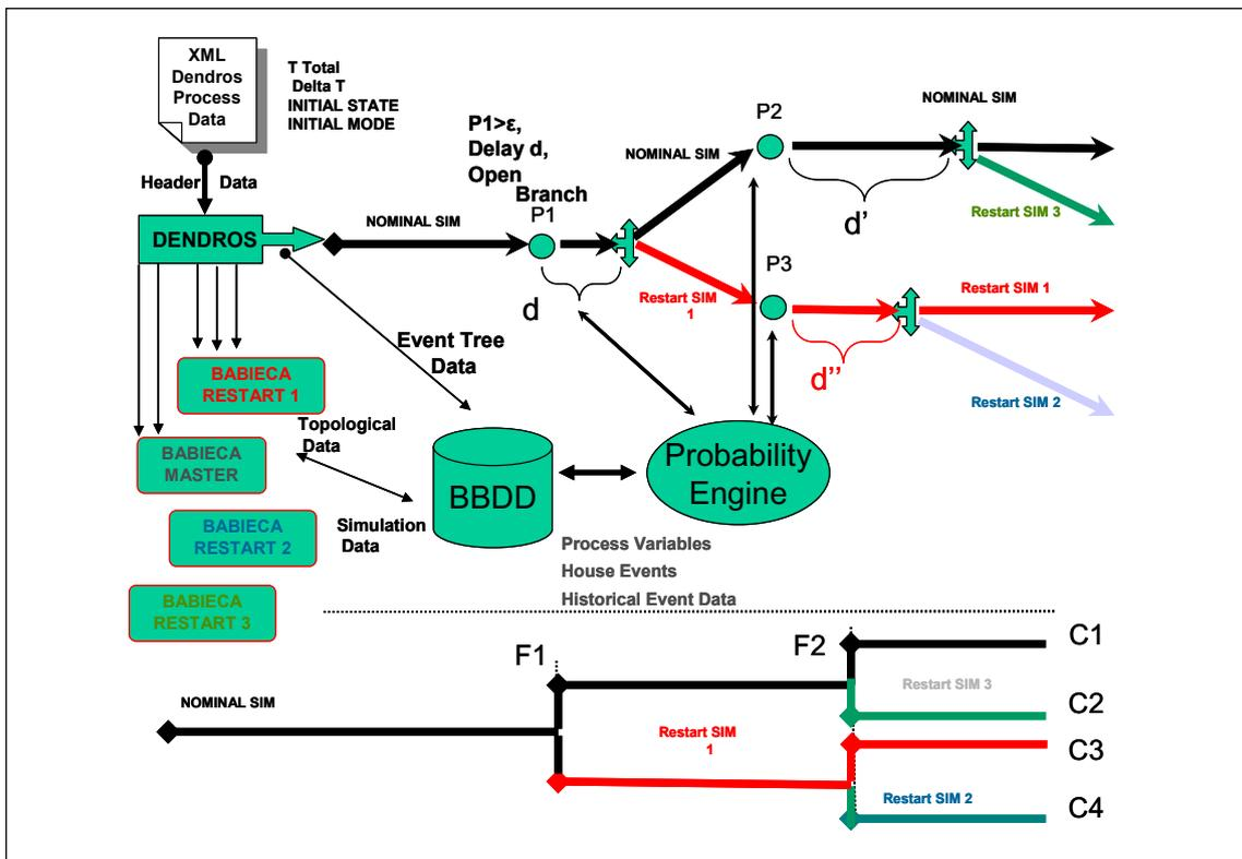
Figure 4. Scheme of SCAIS framework: Simulation of Plant and Operator Actions
