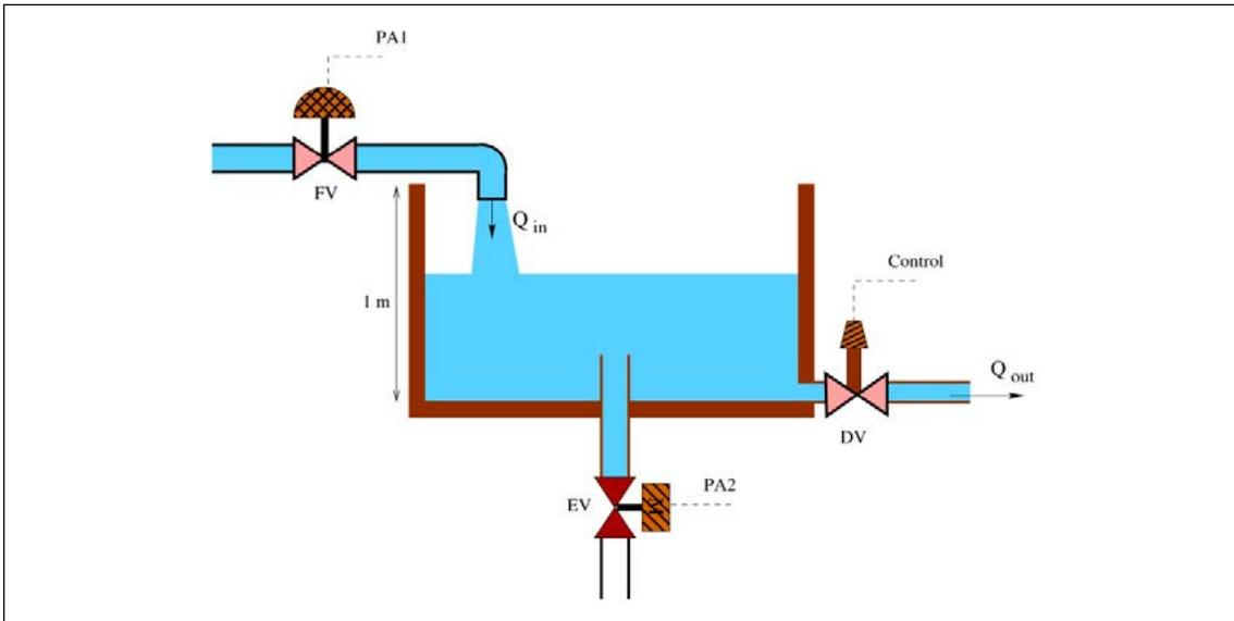
Water is supplied to the tank with volume flow rate  $Q_{in}$ . In normal operation  $Q_{in}$  remains constant. There is also a normal drain line taking water out of the tank at  $Q_{out}$ . A control system is assumed to maintain constant the tank level, i.e.,  $Q_{out} = Q_{in}$  in normal operation. The control system has been assumed perfect and instantaneous and has not been modeled.
