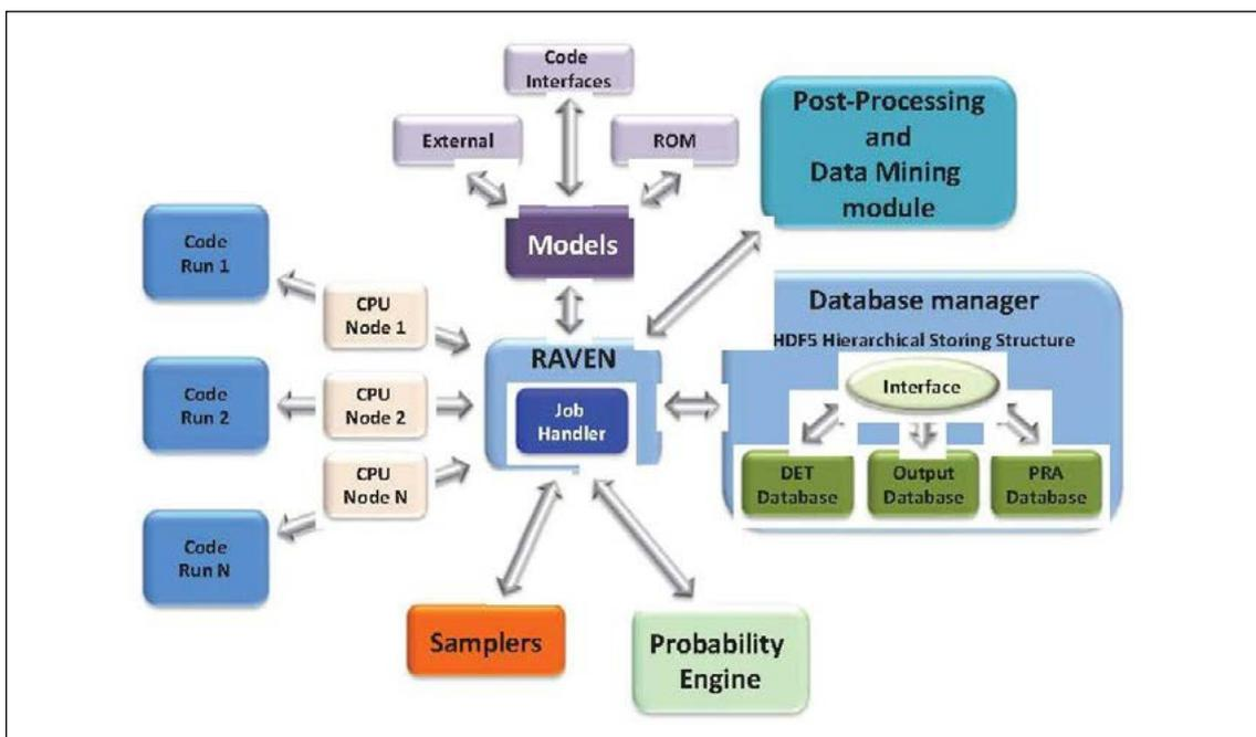
Figure 7. Overview of techniques applied to the 4 main steps of a typical RISMC analysis
