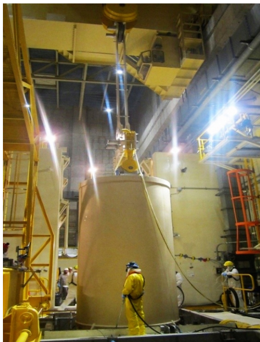
Image of the transfer cask in the fuel building at Ascó.
