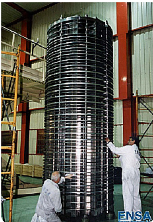
Figure 1. ENSA-DPT container internals: cooling discs and frame
