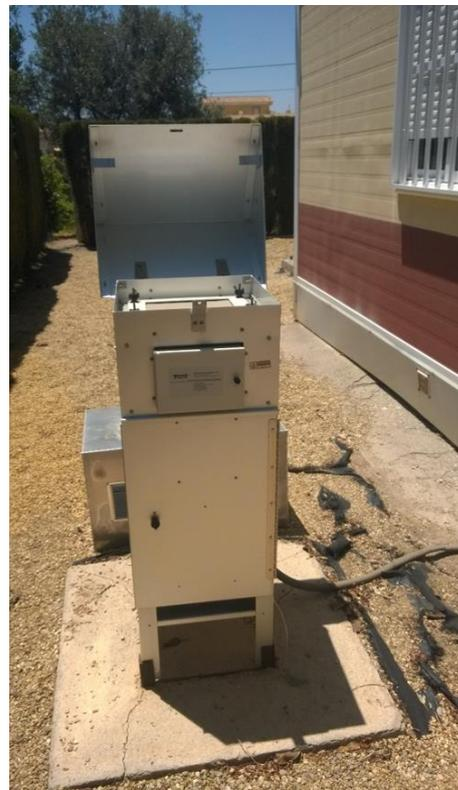
Figure 10. CIEMAT medium volume air sampler
