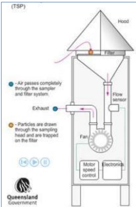
Figure 9. Working scheme of TSP MFC sampler
