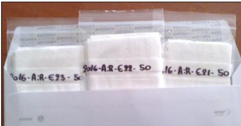
**Figure 19. Air filters in zip lock plastic bags prepared for transportation**
