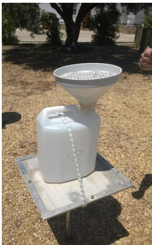
**Figure 11. Atmospheric deposition collector**
