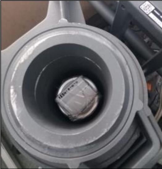
**Figure 20. Air filter ready for measurement by gamma spectrometry**
