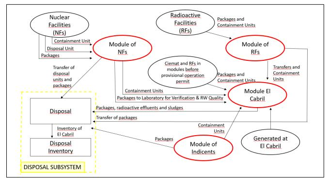
Figure 3: Modules for compiling the radioactive waste inventory
