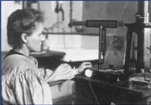
Marie Curie taking measurements with a piezoelectric quartz electrometer
