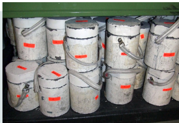
Reusable packages for the transport of radioactive material.
