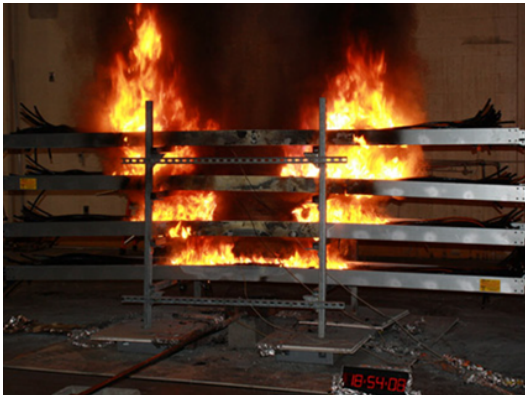
High Energy Arching Fault Testing
